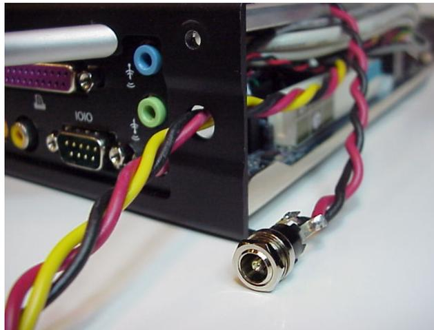
**Figure 13 Removing the existing C134 Power Connector**
