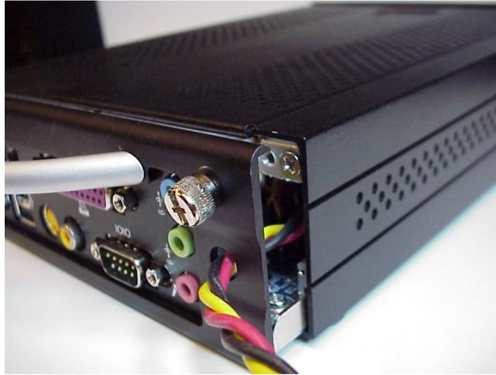
**Figure 9 Opening the C134 Case**
