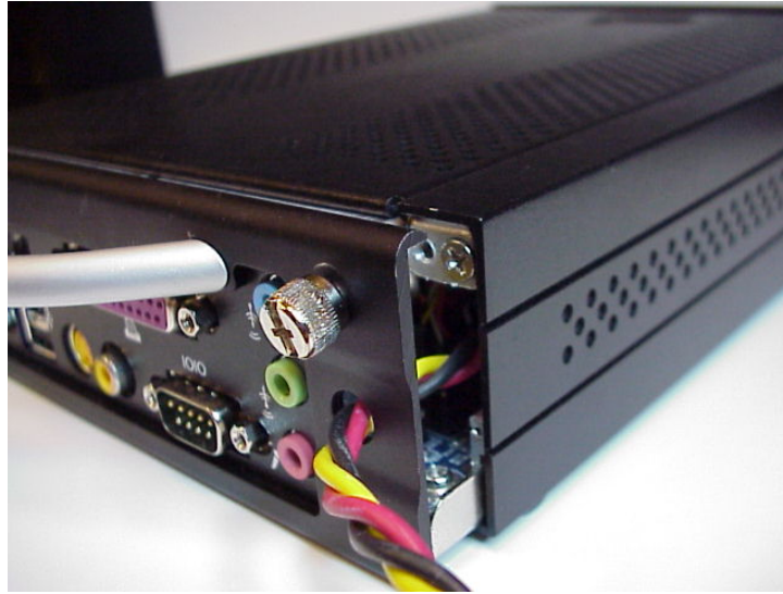
Figure 9 Opening the C134 Case
